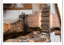
This is the lower horizontal shaft of the sack hoist system. The small horizontal shaft is driven by a large gear wheel on the main verticle shaft.
