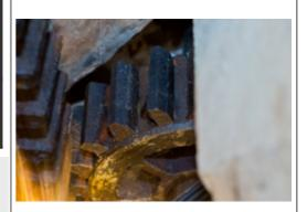
The small gear wheel on the right is the gear wheel which is lowered manually to allow the Mill Wheel to drive the water stones.
