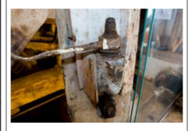
This is the Tentering Up handle of the water-driven stones, one of the two "tentering" handles which are used to alter the height of the beam which lifts or lowers the top milling stone. This action changes the grade of flour being produced.
