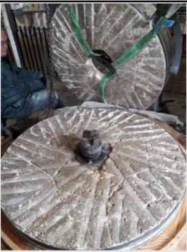
Firstly we strip down the water stone and clean all parts. Then with great care we have to disassemble the stone crane and move it to its new position and then reassemble it. The crane arms are then attached to the stone and the lifting
